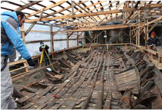
Figure 1. Total Station survey at a Yenikapı Shipwreck (IU Yenikapı Shipwrecks Project Archive).
