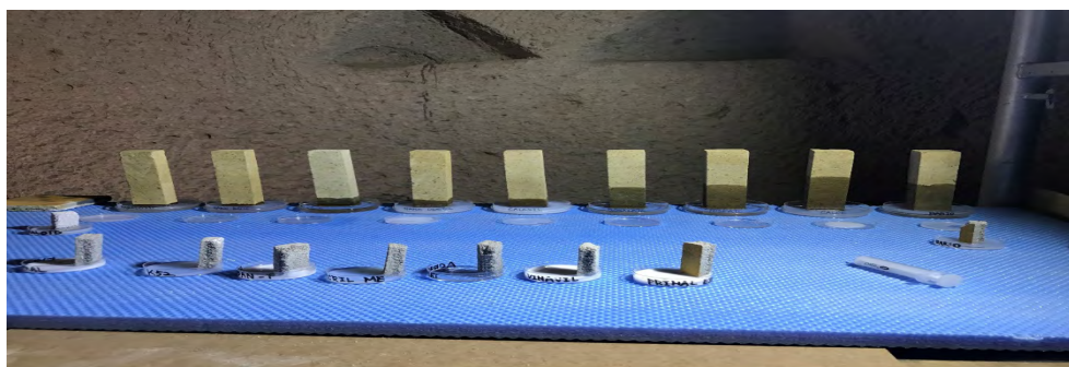
Figure 12. Experiments for monitoring the absorption levels of known consolidation types in building stone tuffs in Tagar Church (Cappadocia, Türkiye) within the scope of the Emergency Response Training Project on Murals carried out by Turkish, Italian, and Japanese conservation experts between 2017-2019 (photo by Şener, 2018).
