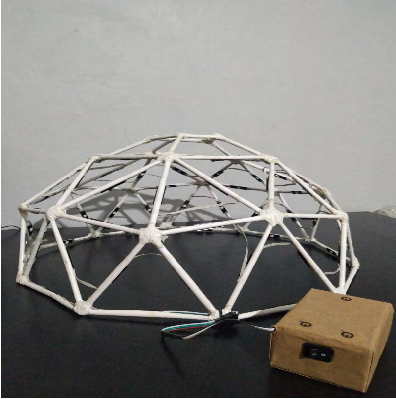
Figure 10. RTI dome in the geodesic structure. (Photo. Emirhan Çetinkaya)
