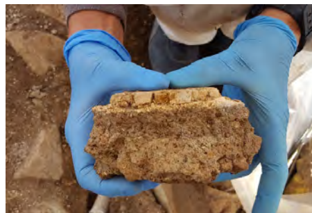
Figure 2. Mosaic fragment showcasing its layered structure, consisting of the following components: tessellatum, bedding layer, nucleus, and rudus.
