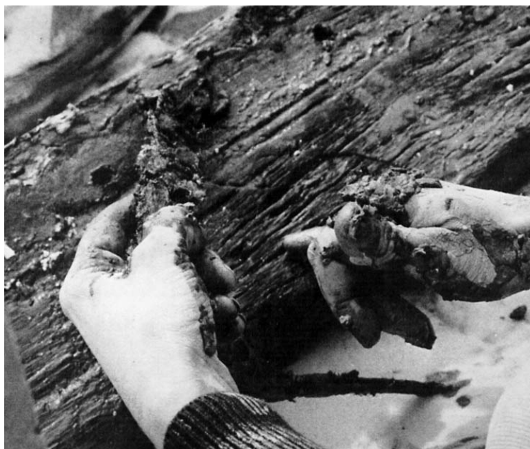
Figure 9. Luting of animal hair pierced by clench-nails (Evans, 1971, p. 114).
