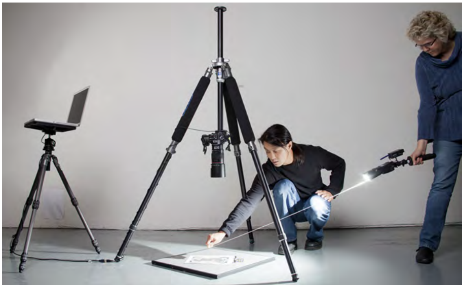
Figure 5. RTI shooting without fixed hardware. (Schroer, 2012)
