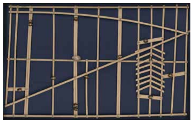
Marshall Islands Stick Chart. A rebbilib (stick chart) from Majōl (the Marshall Islands), circa 1920. The placement of the coconut fibers and shells indicates the location of islands, waves, and currents. The stick charts are the earliest known system of mapping ocean swells in the world. Retrieved from Library of Congress Geography and Map Division, http://lccn.loc.gov/2010586181
